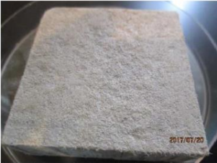
Figure 1. Plycem Structural Flooring Sample 1 Post Incubation.
