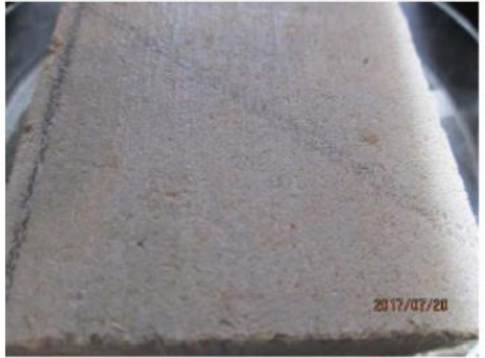
Figure 2. Plycem Structural Flooring Sample 2 Post Incubation.
