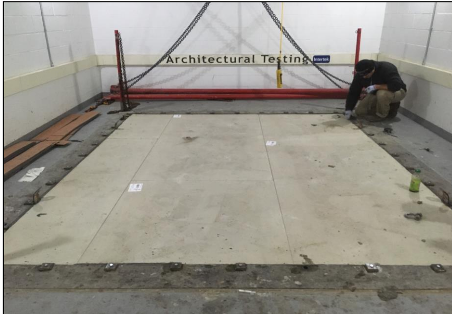
Source Room View of Test Specimen Installation
